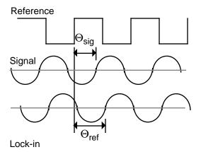
The SR850 amplifies the signal and then multiplies it by the lock-in reference using a phase-sensitive detector or multiplier. The output of the PSD is simply the product of two sine waves.
