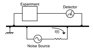
In this illustration, the detector is measuring the signal relative to a ground far from the rest of the experiment. The experiment senses the detector signal plus the voltage due to the noise source's ground return current passing through the finite resistance of the ground between the experiment and the detector. The detector and the experiment are grounded at different places which, in this case, are at different potentials.
