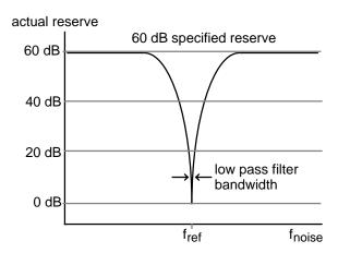
The above graph shows the actual reserve vs the frequency of the noise. In some instruments, the signal input attenuates frequencies far outside the lock-in's operating range (f<sub>noise</sub>>>100 kHz). In these cases, the reserve can be higher at these frequencies than within
